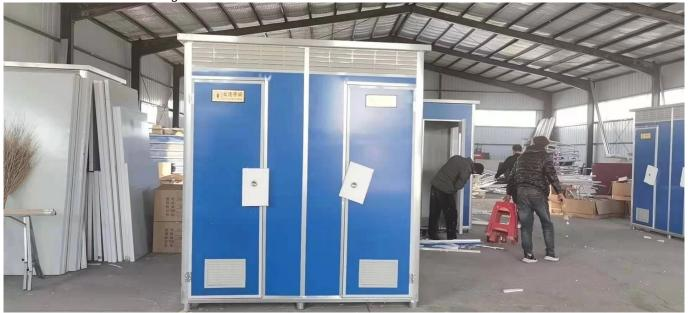
The smaller size <u>prefab toilet</u> is light enough to be easily carried by two people. Very easy to be installed, 2 people can finish one unit within 30 minutes. With flap, the waste can not be seen directly. With vacuum forming, the roof is flexible enough to prevent damage from outside force. With UV-resistance, the toilet can keep its original appearance and function after many years.
